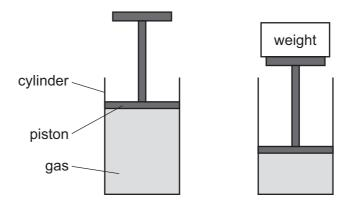
A weight is put on the piston. The volume of gas supporting the piston decreases but the temperature of the gas is unchanged.
