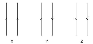
For each pair of wires, what are the forces between the wires?
