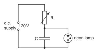
The neon lamp lights when the p.d. across the capacitor C reaches 110 V. C then discharges through the neon lamp. When C has discharged, the lamp goes out and the p.d. across C slowly increases once more.
