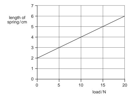
A load causes the spring of the balance to extend by 3 cm.
