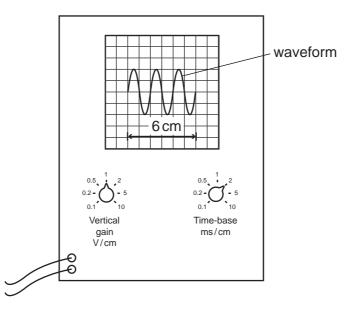
What is the time taken for one cycle of the waveform?
