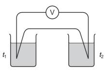
What are the values of  $t_1$  and  $t_2$  when the thermometer is calibrated at the steam point?
