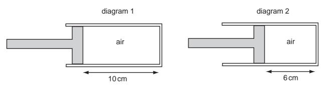
What is the pressure of the air in diagram 2?
